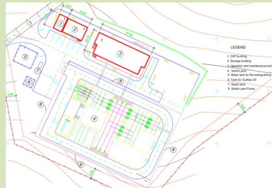
Photovoltaic power plant substation 110kV
