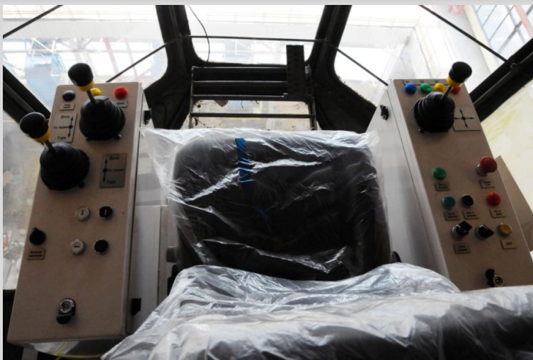
Cabin and control unit of Q=200/32/5t crane
